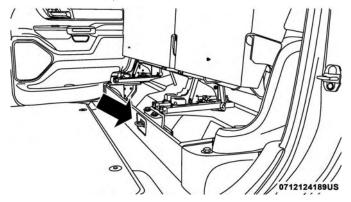
Rotate Lock Mechanism
