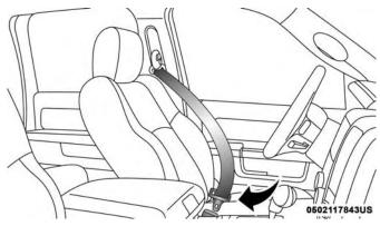
**Inserting Latch Plate Into Buckle**
