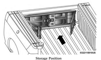
3. Rotate the side gates closed allowing the outboard ends to be positioned in front of the cargo tie down loops.
