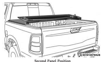
6. Completely unfold the Tonneau Cover.
