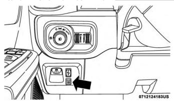
**Instrument Panel Power Inverter Switch**
