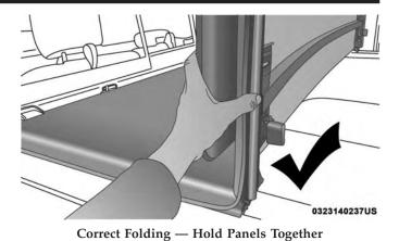
NOTE: Unfold the panel gently. It is not recommended to allow the panels to drop under their own weight.
