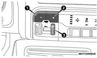
**Integrated Trailer Brake Module (ITBM)**
