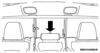
Center Tether Anchorage Over Head Rest
