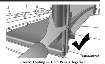
**NOTE:** Fold the panel gently. It is not recommended to allow the panels to drop under their own weight.
